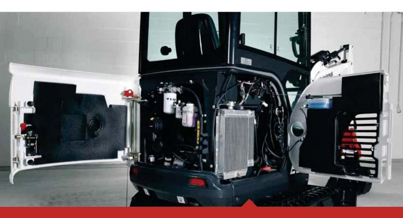
Side-by-side coolers for easy cleaning. Diagnostics are easy thanks to display error codes on control panel and service tool connection. The E20 tailgate provides great access to all daily maintenance components and service points.
