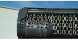
Front rollers allow attachment to better traverse uneven terrain while reducing operator fatigue. Standard equipment on all Brushcat rotary cutters.
