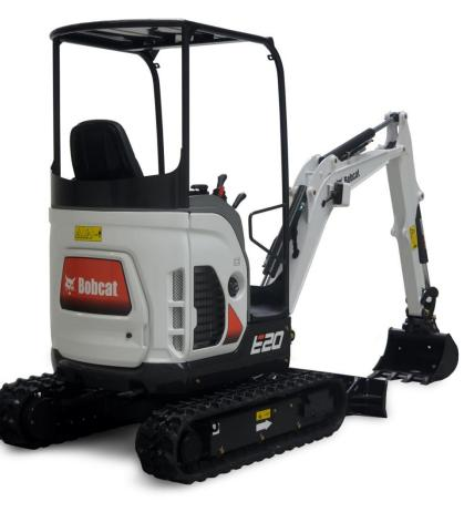
The Zero House Swing (ZHS) concept enhances Zero Tail Swing (ZTS) functionality by further protecting the upper structure corners turning within the swing circle. ZHS functionality provides 320° of free rotation while working close to any object.
