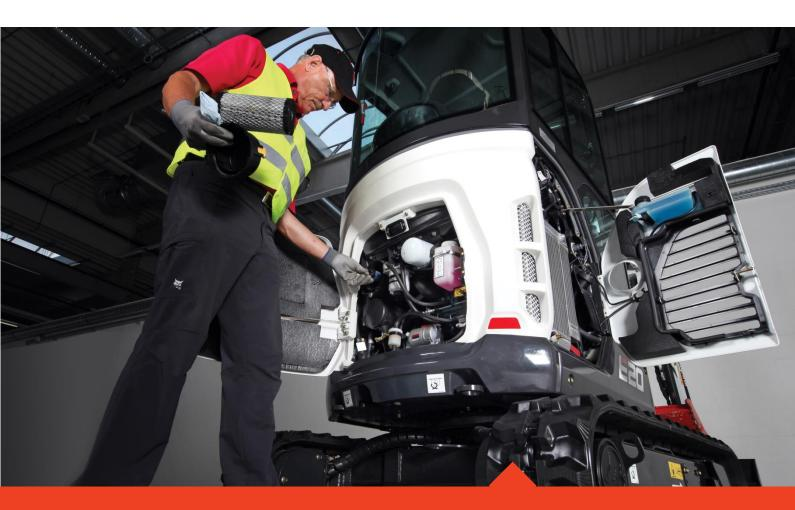
Side-by-side coolers for easy cleaning. Diagnostics are easy thanks to display error codes on control panel and service tool connection. The E20 tailgate provides great access to all daily maintenance components and service points.
